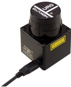
Figure 16: URG-04LX-UG01 LIDAR made by HOKUYO
