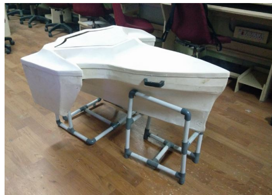
Fig. 4: Fabricated hull and top
