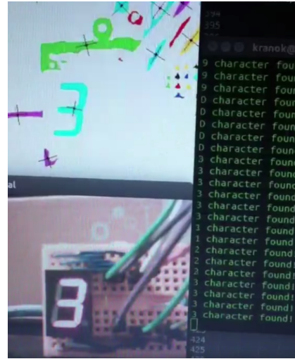
Fig. 8. Testing of number detection using Hu moments.
