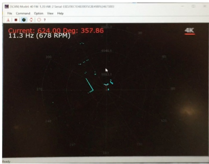
Fig. 7. 2D map generated with the RPLIDAR.
