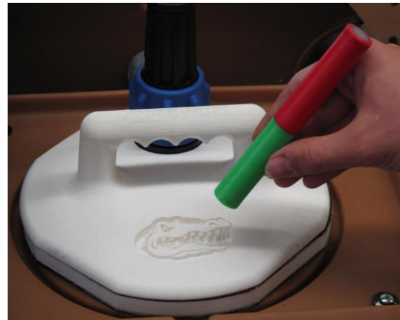
Figure 4: Magnetic kill stick to start the boat (green side) and to stop it (red side).
