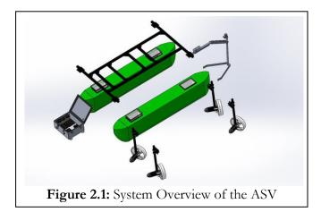
At a high level, the vehicle was made up of two catamaran-style hulls, a connecting frame, four trolling motors at an angle a box holding all the electronics, and an arm that deployed a host of sensors for the acoustic pinging and underwater light challenge.
