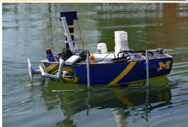
Fig. 7. The electrical box is recessed down inside the hull and can be accessed via a lid that is flush with the deck.
