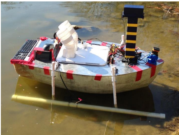
Fig. 4. The hull with outriggers attached
