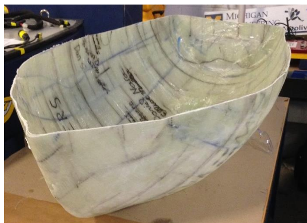
Fig. 3. The finished hull after applying fiberglass to the hullform and removing the foam.
