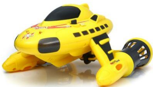
Fig. 6. This is the RC submarine we purchased to modify and use for our AUV.
