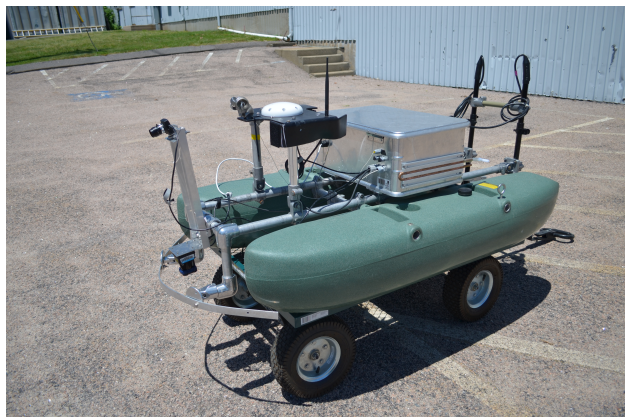
Figure 1: Ram Boat. Vision mounting system is attached to the front of the vehicle with camera and LIDAR. The aluminum cooling fin attached to the side of the vehicle is provides water cooling. No mission specific hardware is attached in this image.
