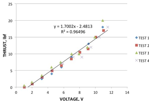
Figure 4: Voltage Versus Thrust Data From Thrust Testing
