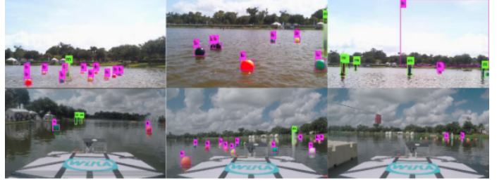
Fig. 4. Detection results from experiment conducted on YOLOv2.
