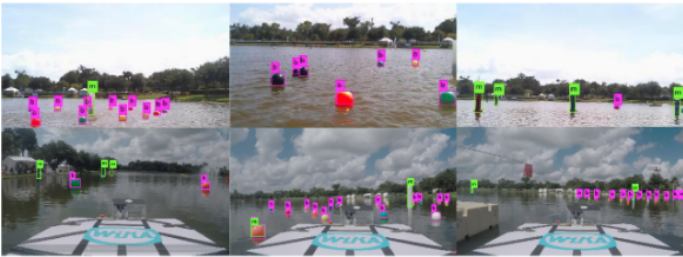
Fig. 7. Detection results from experiment conducted on the lightweight version of Tiny YOLOv3.
