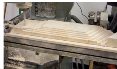
Figure 4: Milled balsa wood pontoon mold
