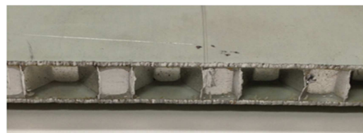
Figure 3: Side view of the aluminum honeycomb deck
