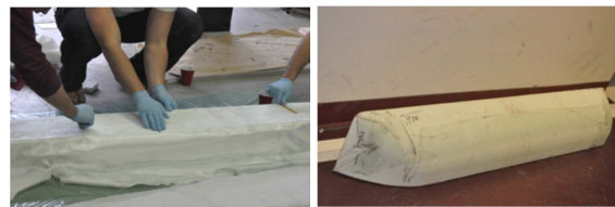
Figure 2: Pontoons shown during and after the fiberglassing process
