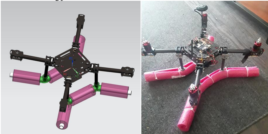
Figure 3. Drone CAD representation vs actual design.
