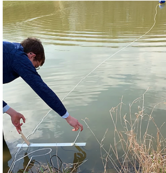
Figure 6: Early Hydrophone Array testing
