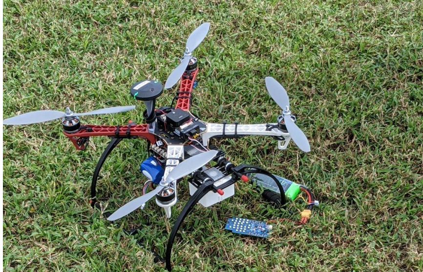
Figure 7: Picture of the quadcopter, having landed directly over the IR beacon in a test.
