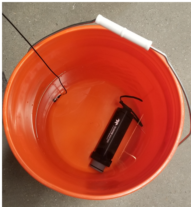
Figure 5: Testing hydrophone circuitry.
