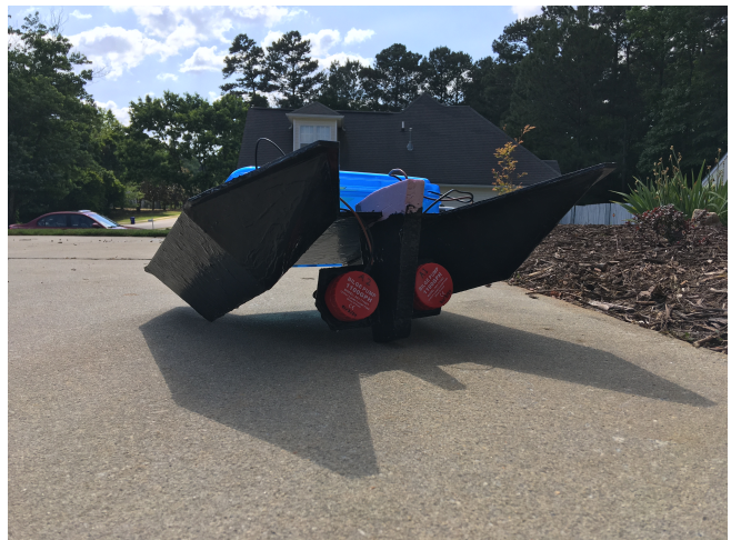
Figure 2: Front view of catamaran, with thrusters.
