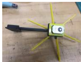
Fig. 11. Fully constructed paddle wheel assembly
