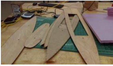
Fig. 3. Laser Cut Wood Templates
