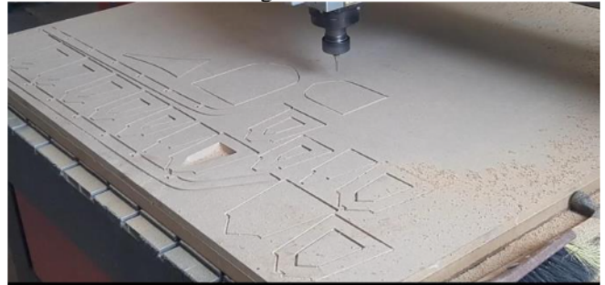
Figure 4: Cutting hull frames using CNC
