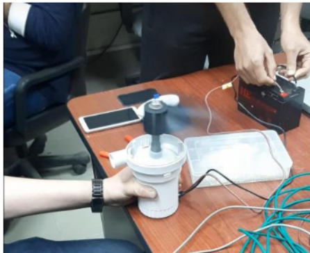
Figure 13: testing a propeller and a pump before using them on the hull.
