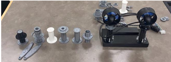
Figure 7 – Thruster mount prototypes from oldest (left) to newest attached to bridge (right)
