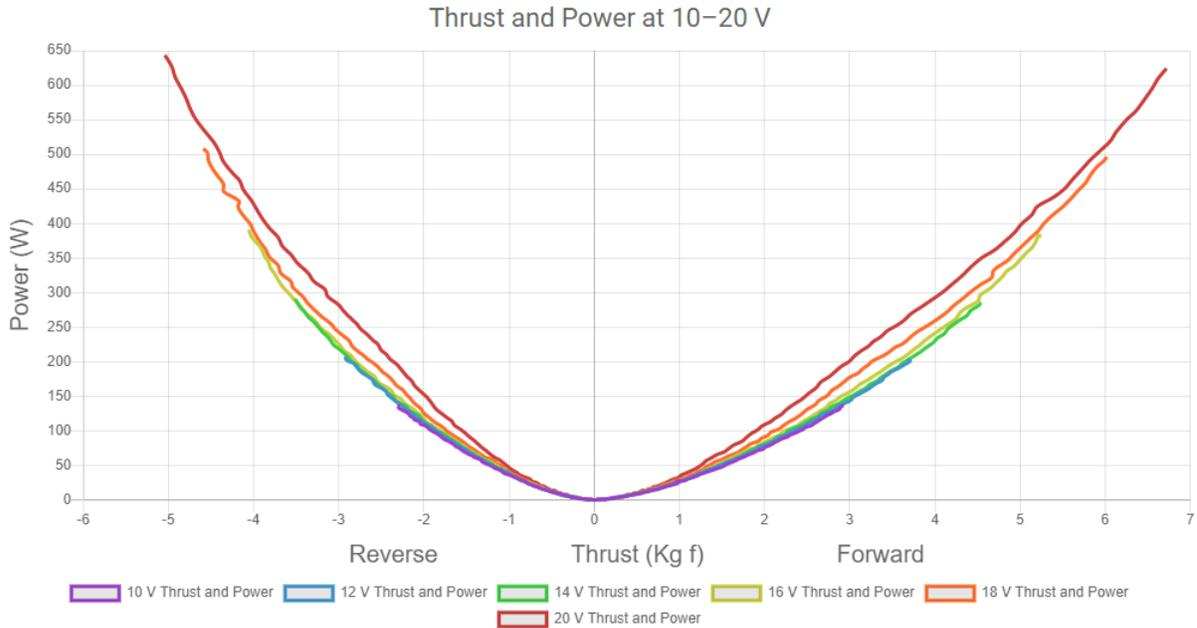
Figure C- 1 T200 Thruster Engine Power Chart
