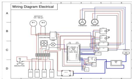
Figure 2. Wiring Diagram Electrical
