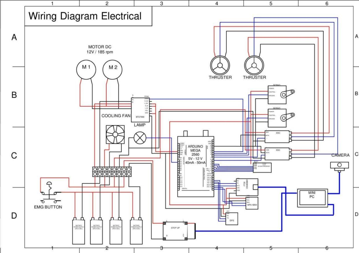
Figure B. 1 Electrical Diagram
