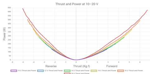
Figure 4. T200 Thruster Engine Power Chart
