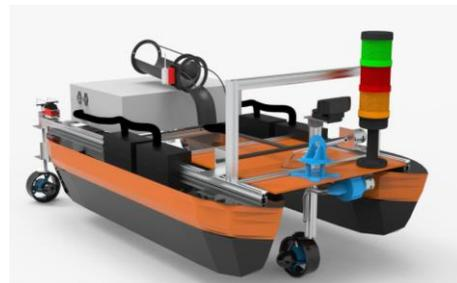
Figure 1. Design of MRT PURVI EVO
