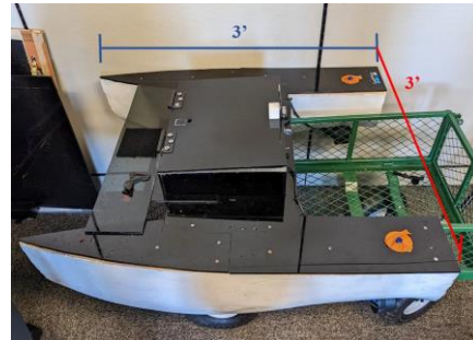
Fig. 1. The autonomous surface vessel's physical design and dimensions.
