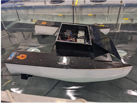
Fig. 5. Weight testing the ASV with 6 kg placed in the bow.
