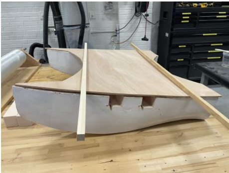
Fig. 6. New plywood deck design.
