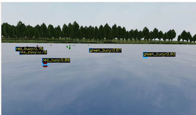
Fig. 4. Performance of the neural network model in real-time buoys detection during the simulation testing
