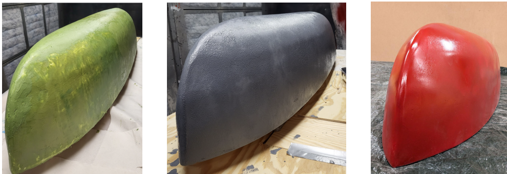
Figure 15: Fairing Compound Coat (L), Barrier Coat (C), Red Paint (R)
