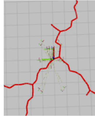
Fig. 7. RRT path planner branching out while looking for a suitable path.
