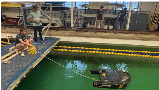
Figure 7. In-Water Testing at the MHL Tow Tank
