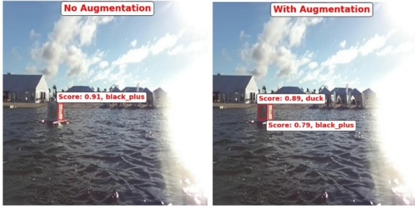
Fig. 4: Comparison of vision detections with and without augmentation in the strong sun
