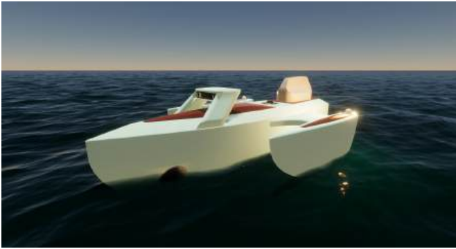
Fig. 9: Illustrates Digital Twin of the Triton in a Unity based ROS2 simulator.
