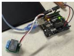
Fig. B.1. Pololu relay module unit test
