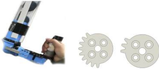
Fig. B.4. Hand-held racquetball launcher (left). There were nine gear teeth in the original configuration (middle), which was revised to three teeth after testing (right).
