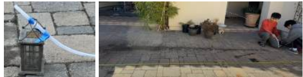
Fig. B.2. First test of water gun without a nozzle (left) and second test with nozzle installed on water gun (right)
