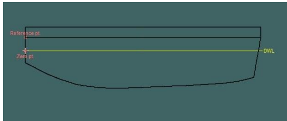
Figure 6. Design waterline of the Boat
