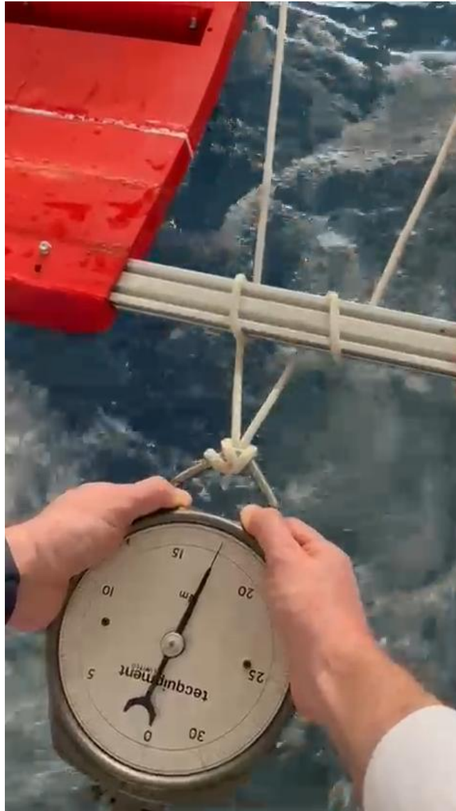
Figure14. Thrust Test @ 24V
