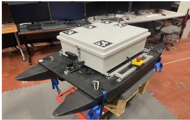
Figure 1. Bayou Bot ASV for 2025 RoboBoat competition
