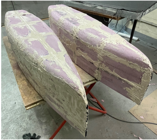
Fig. 4. The two twin pontoons after the skeleton is layered with XPS foam, before fibreglassing. Spray foam is used to seal any gaps.
