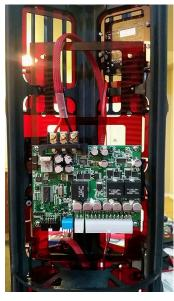
power for our computing systems. This power supply provides a standard ATX power connector for the motherboard as well as regulated 5V and 12V supply Propulsion rails. systems are powered with unregulated power from the power distribution board.
