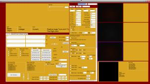
The mission planner is unique in that it is built in modules with the ability to select which missions to run and in what order. The Command Interface also allows on the fly changes to particular missions ranging from motor control multipliers to disabling parts of the mission altogether.
