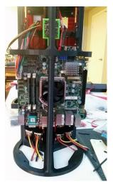
peripherals. A Phidgets interface kit is used for GPIO and Analog to Digital Conversion. A CAT5 KVM extension system is used to enable tethered programming and control
