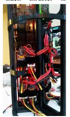
remaining actuation systems are controlled by a Phidgets 4 Channel relay module.
