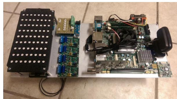
Figure 6: Main electronics rack with all components mounted, prior to wiring.
