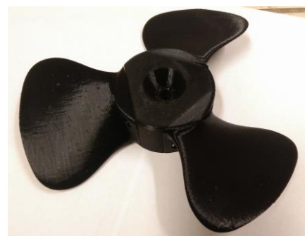
Figure 5: 3D printed bi-directional propeller.
