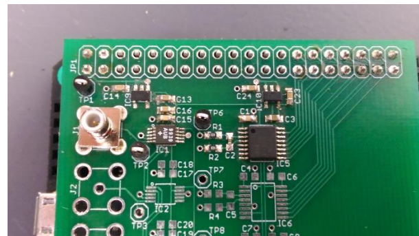
Figure 8: Single channel of localization board. The 10-pin TSSOP is a MAX9939 programmable gain amplifier, and the 16-pin SOIC is an ADS8327 16-bit ADC.
