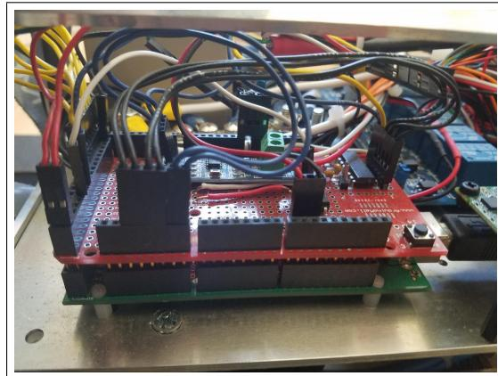
Figure 5: Atmega2560 Microcontroller
