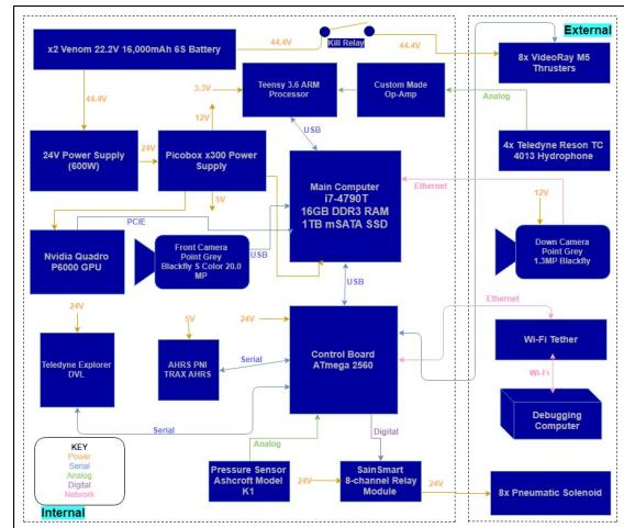
Figure 4: Overview of Marlin's electrical system
