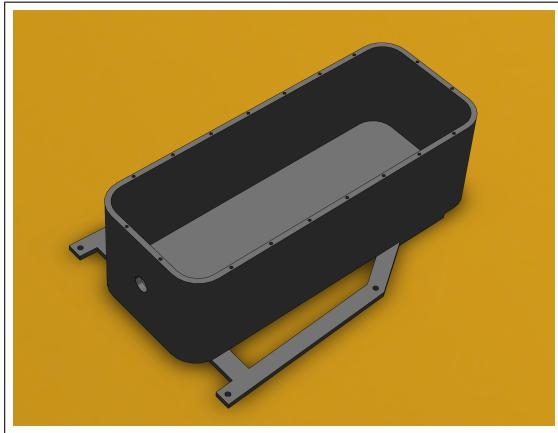
Figure 3: DVL Mount modeled in Solidworks
