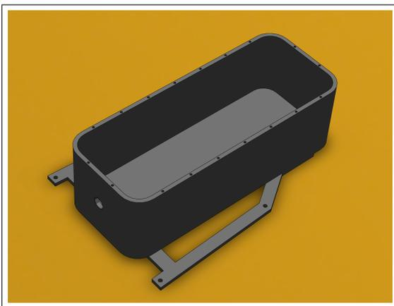
Figure 3: DVL Mount modeled in Solidworks
