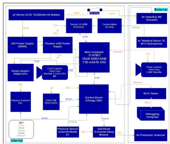
Figure 4: Overview of Marlin's electrical system
