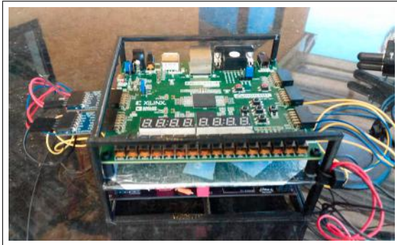
Figure 7: FPGA with hydrophone circuits
