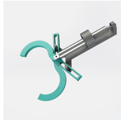
Figure 6. Prospero Mark II's Pneumatic Gripper
