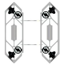
Fig 3. Prospero's final thruster layout.
