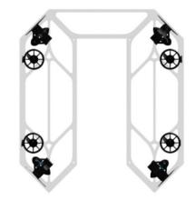
Fig 4. Prospero's second thruster layout.
