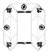
Fig 2. Prospero's initial thruster layout.
