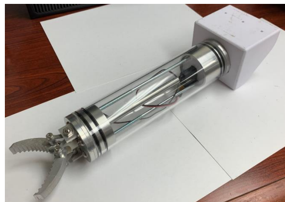
Figure 4: Assembled mechanical arm for installation on GY4R4D0S.
