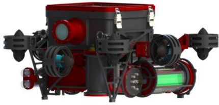
Fig. 1: Ajax's biggest design innovation is its innovative small yet functional frame. It features support for more external enclosures than ever before as well as dedicated room for trimming foam while having one of the smallest profiles to date. The electrical system is also almost identical to Odysseus.
