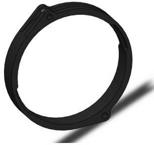
Figure 7. Auxiliary enclosure mounting brackets designed in SolidWorks.
