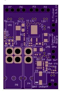
Figure 8: Computer Side Power PCB
