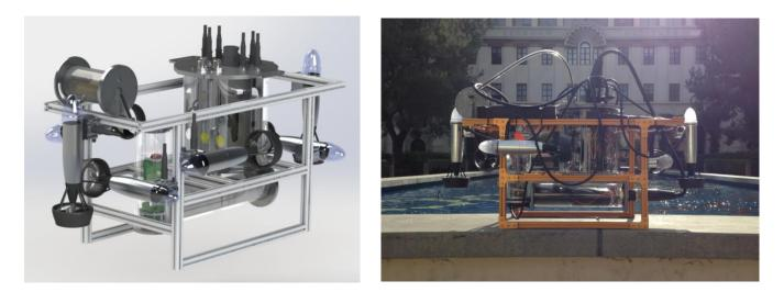
Figure 1: CAD Model and photograph of the Completed Vehicle
