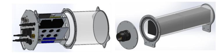
Figure 4: Pressure Hull Design
