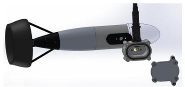
Figure 3: Custom Mounting Scheme for VideoRay Thrusters
