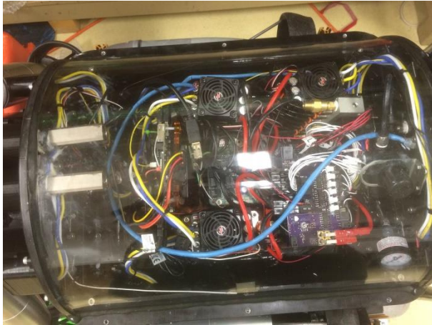
Fig. 5. The electronics inside the hull. The thrusters are mounted directly to the main pressure hull so that no underwater connectors are needed.
