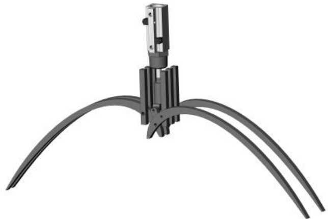
Fig. 4. The gripper is actuated by a pneumatic cylinder located above the gripper mechanism.
