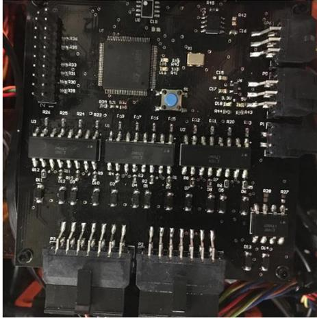
**Figure 8: Pneumatics board.** Optoisolated GPIO signals control pneumatic solenoids which actuate the torpedoes, markers, and grippers.
