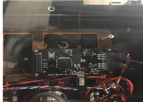
**Figure 6: Core board.** This standalone board handles communication between the Intel NUC™ computer and the rest of the microcontroller system.
