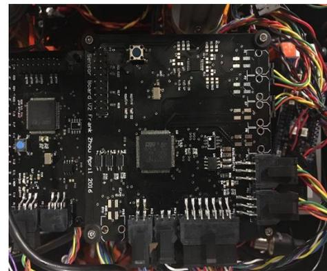
**Figure 7: Sensor board.** The sensor board polls the depth sensor, motor kill switch, and controls the feedback LED strips.
