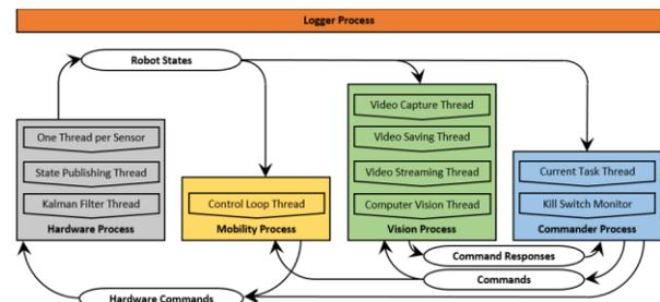
**Figure 9: Software architecture.** The five main processes that run on the vehicle and the interprocess communication channels are shown. Each process is illustrated by a large box, with threads inside. Each circular box represents a communication channel.
