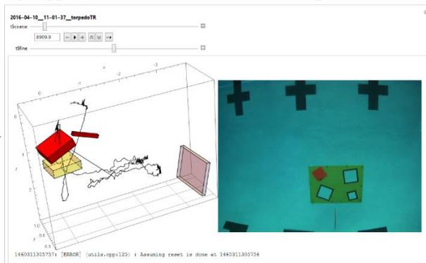
**Figure 10: Log file analysis GUI.** The GUI displays the vehicle's position and gimbal orientation (red), the target state (yellow), the complete vehicle path, the detected object, and the camera image.
