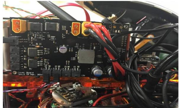
**Figure 5: Motor power board.** The upper left contains the protection circuitry while the rest of the board contains voltage regulators. The board is modular in that they can power the motors or the computer depending on which components are soldered on.
