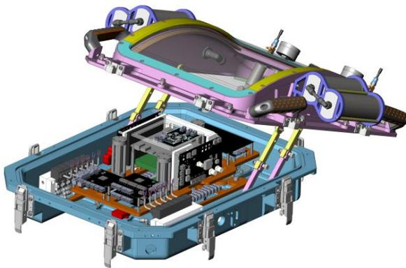
**Figure 2: Main pressure hull.** The four-bar linkage keeps the top connected to the bottom when open. The top electronics platform rises to provide convenient access to the boards below.
