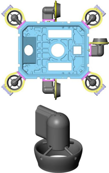
**Figure 3: Thrusters and thruster configuration.** The thruster configuration (top) uses seven VideoRay M5 brushless thrusters (bottom). The thruss for Dory (above)). The configuration consists of four vertical thrusters, two forward-facing thrusters, and one lateral thruster.
