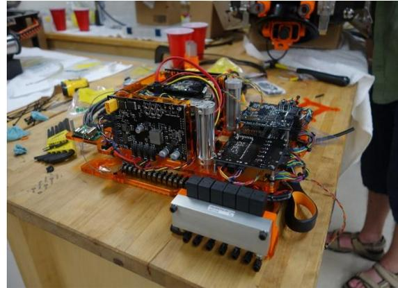
**Figure 4: Electronics package outside the pressure hull.**
