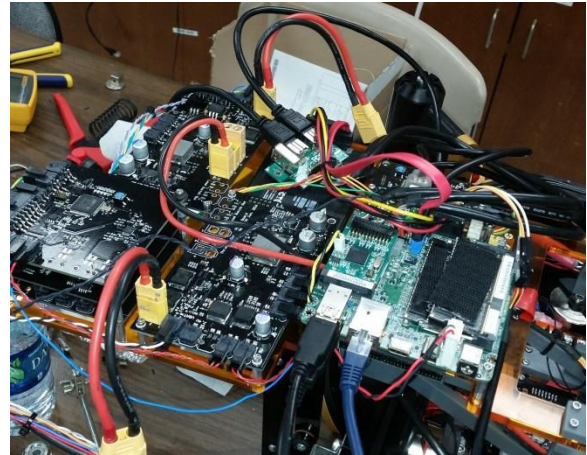
Figure 7: Flo's electronics package outside the pressure hull.
