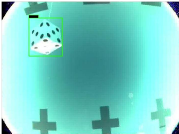
Figure 17: The you-only-look-once model's bounding box prediction. The green box is the model's prediction of the region-of-interest, i.e. where the object is thought to reside within.
