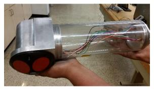
KVH DSP-1750 single axis Fiber Optic Gyro
