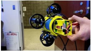
The same type of setup is used for the pneumatics module and the DVL module. The DVL is slightly different in that it has an aluminum fixture on one end so that it could accommodate the DVL head that needs to be in a 90% differential in relationship to the polycarbonate tube that houses the electronics.
