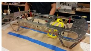
The main hull is made of several sections to allow for future modifications and ease of maintenance. The center section of the main hull is comprised of a  $\frac{1}{2}$ " aluminum tube that has been faced off so that industry standard what tight connectors can be mounted. It acts much like a spine for all the thrusters and external sensors and instruments. On each end of the main hull
