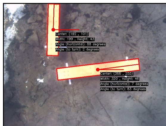
Fig 9. Our Pathmarker detection code running on a video frame. (Test Image Credit: CUAUV Robosub Team)[1]
