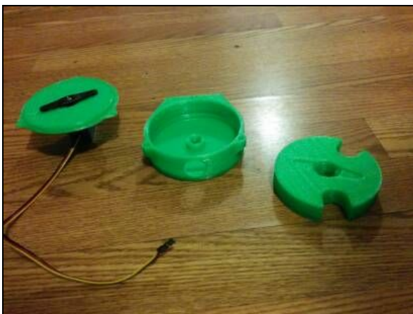
Fig 10. 3D Printed ¼” SS Ball Bearing Marker Dropper Designed by Adam Thorp
