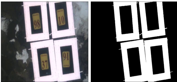
Fig 6. Ground Truth Segmentation images have been generated from available media to allow for improvements in image filter code to be measured. (Test Image Credit: CUAUV Robosub Team)[2][1]
