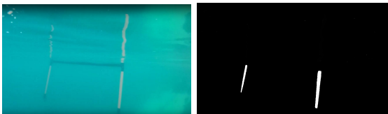
Fig 4. Ground Truth Segmentation images have been generated from available media to allow for improvements in image filter code to be measured. A sample subset has been reserved for validation testing to avoid overtraining. [1]
