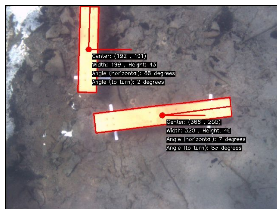
Fig 5. Our Pathmarker detection code running on a video frame. (Test Image Credit: CUAUV Robosub Team)[2][1]
