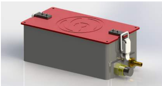
Fig. 8: Thor's battery pod enclosure
