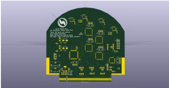
Fig. 10: The serial board implementation featuring the back-plane edge connectors
