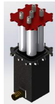
Fig. 17: A SolidWorks rendering of Loki's solenoid valve enclosure
