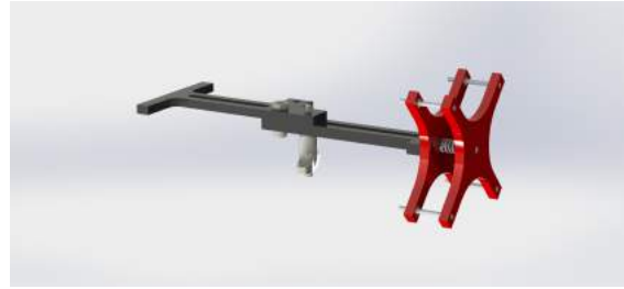
Fig. 6: One of Thor's forward manipulators
