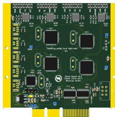
Fig. 13: Rendering of Serial Board. The USB ports are along the left edge with the four FTDI USB to UART interface ICs in the middle of the board and the RS-232 level shifters along the bottom edge directly above the solt-edge connector.
