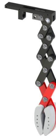
Fig. 7: The downward manipulator parallel linkage arm in its extended state. The links gradually increase in length towards the bottom. The mounting and links are made from 6061-T6 and the gripper (grey at bottom) is 3D printed with ABS plastic.
