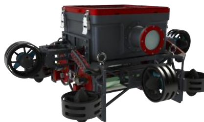
Fig. 3: Pollux's biggest design innovation is the unibody aluminum hull. The secondary vehicle features an identical electrical system to the main sub in a much smaller form factor.
