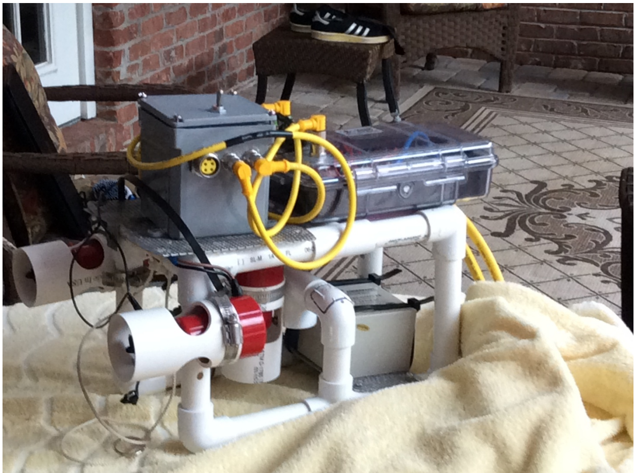
Figure 6 Our Sub With the PVC Frame Holding the Brains
